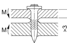
To prevent imposition of a moment on the shank of fastener, use three fasteners in a group.
