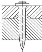
If a gap between the fastened part and the base material is unacceptable, the fastened part needs to be prepared with drilled holes.
