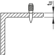
Steel thickness:  $t_{II} \geq 6 \text{ mm}$
