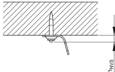
$$h_{NVS, \min} = 6 \text{ mm}$$
