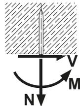
Note: If relevant, prying forces need to be considered in design, see example. Moment acting on fastener shank only in case of a gap between base and fastened material.
