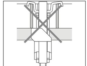
The saddle of the fastener should not be bent, see installation instructions below.
