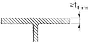
For beams with composite decking:
