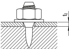
$$t_I \leq L_g - t_{\text{washer}} - t_{\text{nut}}$$
