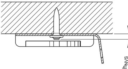
$$h_{NVS, \min} = 3 \text{ mm}$$
