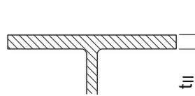
$t_{II} \geq 4.0 \text{ mm}$  (for nail)
