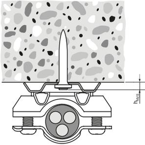
$$h_{NVS, \min} = 3 \text{ mm}$$
