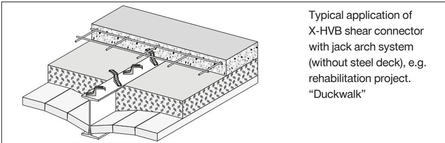
Typical application of X-HVB shear connector with jack arch system (without steel deck), e.g. rehabilitation project. "Duckwalk"
