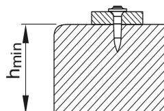
Concrete:  $h_{min} = 80 \text{ mm}$
