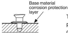
Thickness of base material corrosion protection layer  $\leq 0.4\text{mm}$ . For thicker coatings, please contact Hilti.
