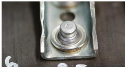
Clearly visible piston mark on top washer
