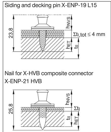
Guide values for the depth of penetration of specific fastener types are as follows:
