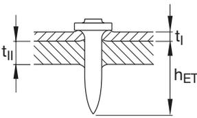
For standard fastening:  $L_s = h_{ET} + t_I$
