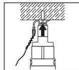
4. Locate the nail, compress the tool, pull the trigger and the fastening is complete
