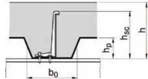
x)  $b_o/h_p \geq 1.0$  for composite decking perpendicular to beam combined with X-HVB orientation parallel with beam
