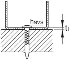
X-S:  $h_{NVS} = 2-4 \text{ mm}$
