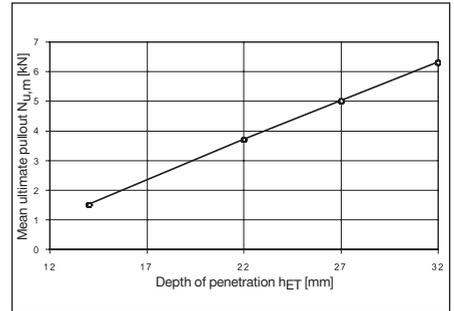
The value of increasing the depth of penetration in order to increase pull-out strength is limited by the increasing fastener driving failure rate. Provided that the penetration depth is the same, fastenings in concrete with a higher compressive strength hold better than fastenings in lower strength concrete. The ability to exploit this
