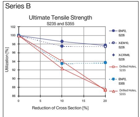
Graphs of the utilization versus cross-section reductions show that:
