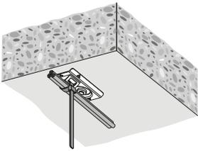
Fastening electrical installation to ceiling and wall
