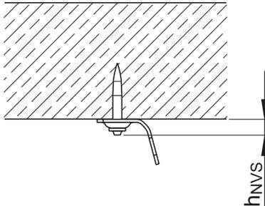
$$h_{NVS, \min} = 6 \text{ mm}$$
