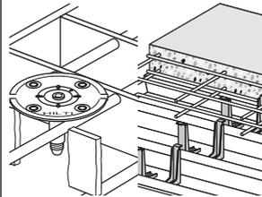
The nails used (also known as drive pins) are of a special type equipped with washers to meet the needs of the application and to provide guidance when driven. Threaded studs are essentially nails with a threaded upper section instead of a head. Composite fasteners are an assembly consisting of a nail with an application-specific fastening component such as a clip, plate or disk made of metal or plastic.
