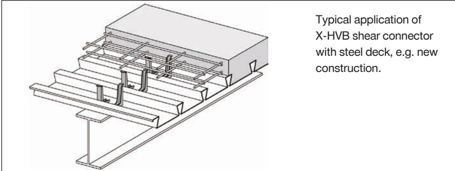
Typical application of X-HVB shear connector with steel deck, e.g. new construction.
