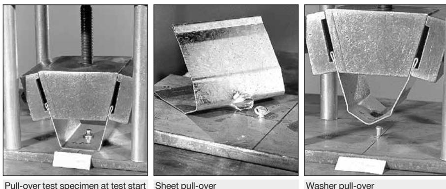
Pull-over test specimen at test start
