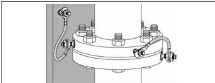
Functional and protective bonding in pipe
