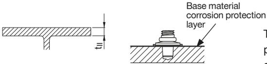
Thickness of base material corrosion protection layer  $\leq 0.4$  mm. For thicker coatings, please contact Hilti.
