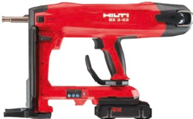
This tool is propellant-free. The energy moving the piston is generated by an electrical motor, two springs and a belt. The only source of energy required is a 22V battery which is interchangeable with other tools from the Hilti 22V platform family.
