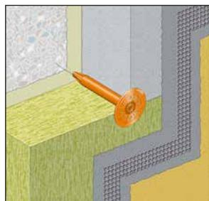
The XI-FV fastener is used to transfer wind suction loads acting on the thermal insulation composite system. The base material is normal weight concrete, which is either uncoated or coated with plaster or tiles. Coatings with plaster or tiles is often met if existing buildings are renovated and are improved with regards to their thermal insulation properties.
